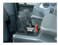
control lever column can be slid forward or backward and the largesized arm rest can be adjusted up or down to provide the operator with a variety of comfortable operating positions.
