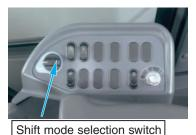
(low and high). The operator can match the machine's operating requirements with opitimum performance efficiency. This system is controlled with a dial on the right control panel.
