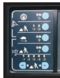
Track Shoe Slip Control Panel
