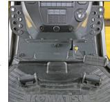
one pedal of decelerator/brake pedal. Operation of pedal function can be changed by the mode selector switch.
