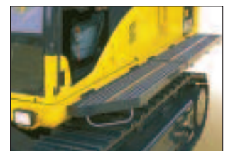
Large Handrail and Wide Catwalk
