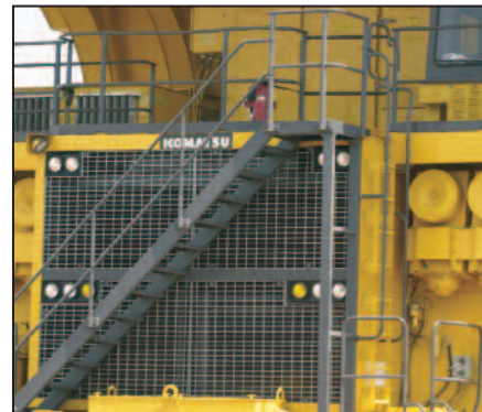
Komatsu's 960E-2K offers stairway access with entry from either the right or left side of the truck depending on the customer's preference.
