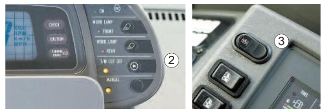
2: T/M cutoff ON/OFF switch 3: T/M cutoff set switch
